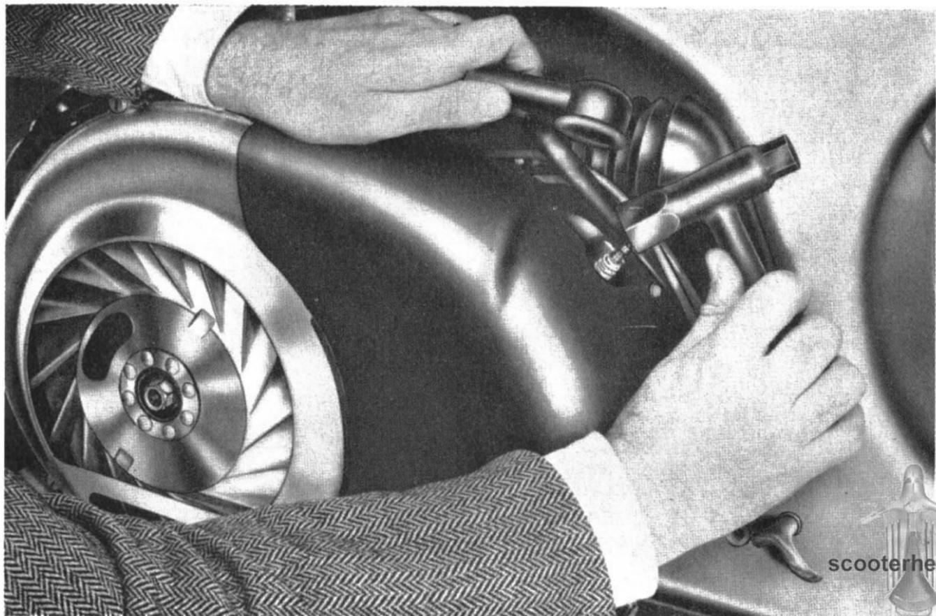
Fig. 14—Removing spark-plug
