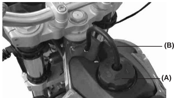
(A). Fuel cap. (B). Fuel vent hose.
