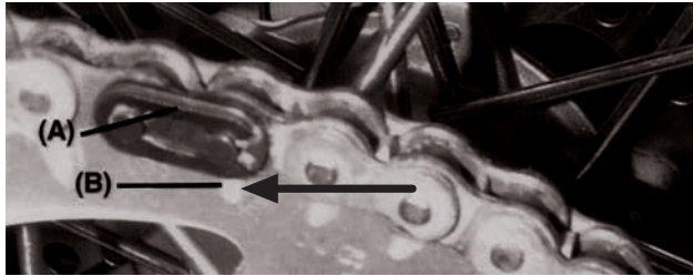
(A). Clip. (B). Chain direction of rotation.
