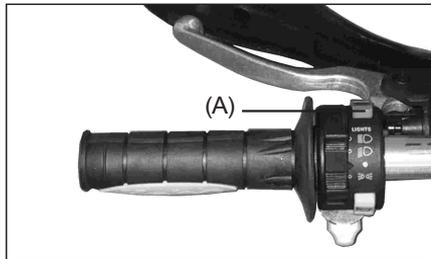
2. After racing the engine slightly, close the throttle completely and push the engine stop button (A).
