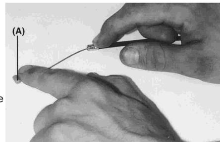
Apply grease to the following point throttle inner cable upper ends.
