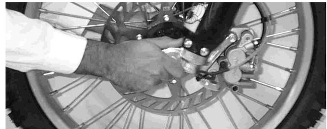
To check the steering adjustment, using a stand under the frame, raise the wheel off the ground. Push the handlebar lightly to either side; if it continues moving under its own momentum, the steering is not too light. Squatting in front of the motorcycle, grasp the lower ends of the front fork at the axle, and push and pull the bottom end of the front fork back and forth; if play is felt, the steering is too loose.
