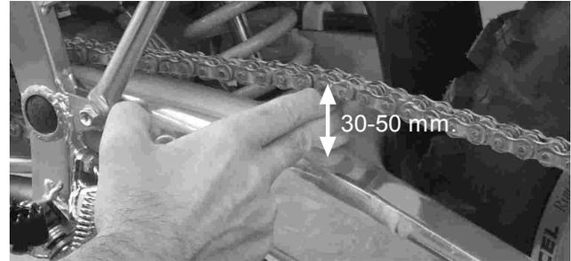
In addition to checking the slack, rotate the rear wheel to inspect the drive chain and sprockets for damaged rollers, loose pin and links, unevenly or excessively worn teet, and damaged teeth.
