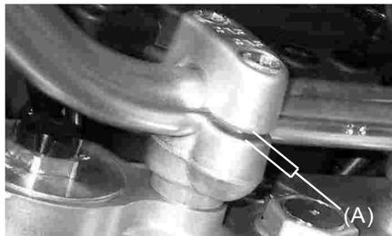
If the handlebar clamp is correctly installed, there will be an even gap at the front and rear after tightening. (A).
