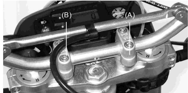
Tighten the clamp bolts, front first and then the rear, to 25 Nm of torque (18 ft.lbs).
