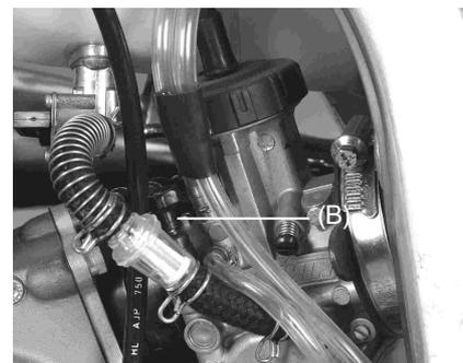
3. If the engine is cold, pull up the choke knob (B).
