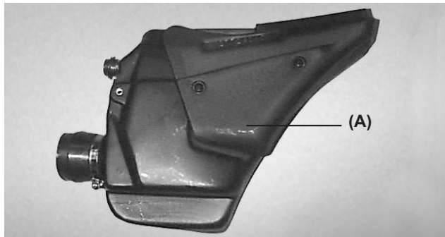
(A). Air filter box.
