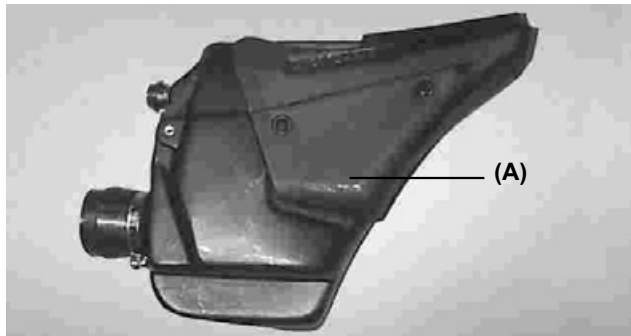
(A). Air filter box.
