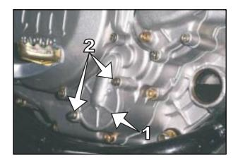
Wait until the oil has been removed completely, then clean the sump and cover surfaces, check the O-Ring and replace it if necessary. Insert a new filter cartridge, making sure that the open side is towards the outside of the engine. The filter must insert into the sump as far as possible in its seat.
