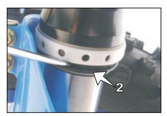
Clean the rdust scraper, the external pipes and the rods carefully. Oil them well with silicone spray or with engine oil. Finally, push the dust scraper manually into the external pipes.
