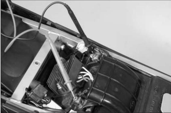
**Regulator rectifier output** – measure the voltage with the measuring leads of the peak voltage adapter directly on the poles of the vehicle battery:
