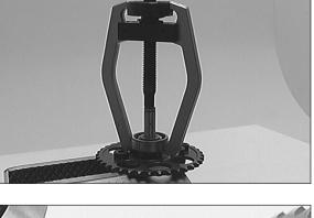
Use the puller tool to extract the grooved ball bearing 6 from the camshaft (see photo).
