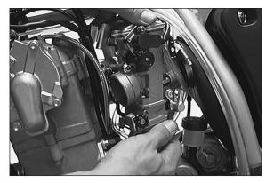
Loosen the 2 hose clamps (3) + (4) and pull the carburetor out of the connection boot.
