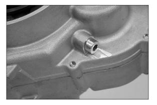
Turn the crankshaft to TDC and mount the crankshaft fixing bolt without a sealing ring.
