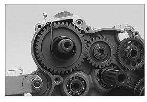
Insert the preassembled kickstarter shaft into the bearing bore such that the ratchet gear is positioned behind the release plate.
