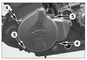
Apply a new gasket and fix the ignition cover with the 4 bolts (4) and
