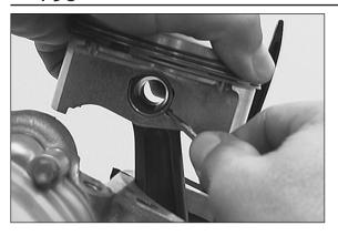
Remove the wire circlip and the push piston bolt from the piston. Dismount the piston.
