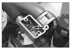
Refill oil, until oil is discharged from the bore **4** of the master cylinder in a bubble-free state. Make sure that the oil does not overflow.
