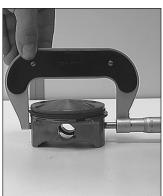
NOTE: The size of the cylinder • is marked on the cylinder, the size of the piston is marked at the top of the piston 2.
