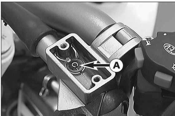
Refill oil, until oil is discharged from the bore ❶ of the master cylinder in a bubble-free state. Make sure that the oil does not overflow.
