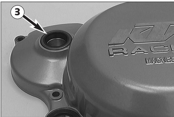
**Clutch cover****Shaft seal ring of kickstarter shaft ③**
