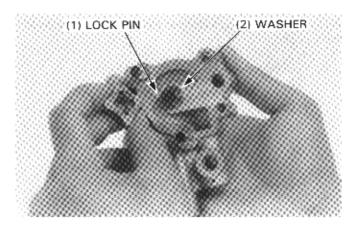
Separate the oil pump body from the oil pump cover B. Remove the following from the cover B.
