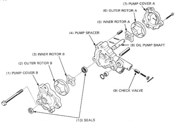
Install the outer rotor B in the oil pump cover B with the punch mark on the rotor facing inside.
