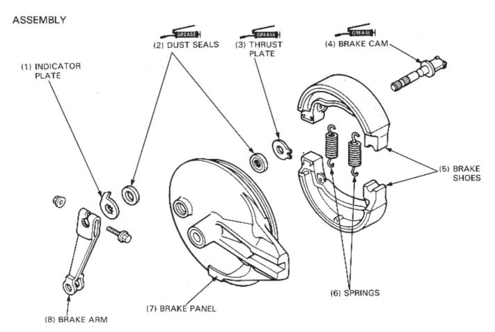
Apply grease to the dust seals, and install them into the brake panel.
