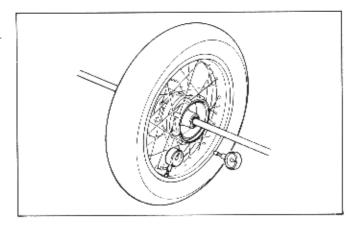
Check the condition of the final driven sprocket teeth. Replace a worn or damaged sprocket.
