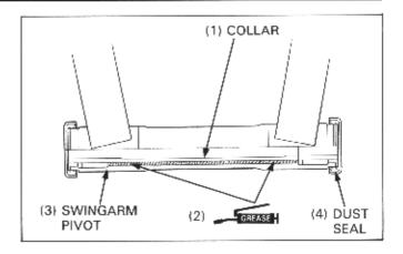
Install the following parts to the swing arm:
