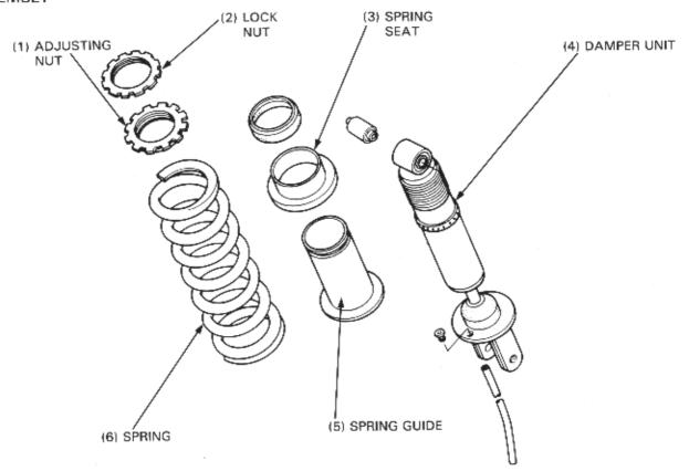
Install the spring, adjusting nut and lock nut.
