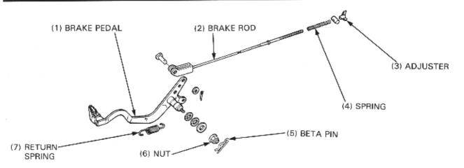
Apply grease to the dust seal lips and brake pedal pivot, and install the brake pedal.
